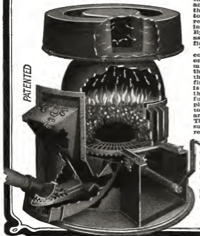
Illustration shows furnace without casing, cut away to show how coal is forced up under fire, which burns on top.
